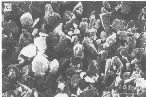
Figure 1 Scanning electron micrographs of oxide powders of (a) cordierite, (b) forsterite and (c) spinel.
